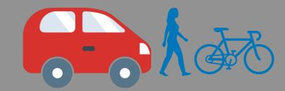
Three hundred milliseconds later, the lidar re-classified her as a bicycle, and determined that it would be impossible at this point to maneuver around her. With just 200 ms until collision, the ADS began braking the vehicle, pitifully too late to stop in time.
